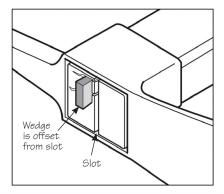
While it is normal for the end of the wedge to stick out from the top of the handle, make sure the head is fixed tightly on the handle before each use; otherwise, the head may come off while working. If the head feels loose, tap the exposed wedge a little deeper into the handle. **Do not** drive the entire wedge into the handle at once, as this will damage the handle.
